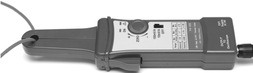
Figure 2: Connecting the PA-622 current probe.
