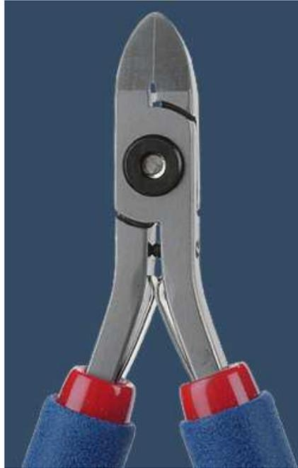
Adjustable anti-dulling protection is provided by a setscrew stop placed either in the handle or jaw of the cutter. The setscrew is adjusted at the factory to stop cutting edge motion exactly as the two blades come together. The setscrew thus prevents the blades from damaging themselves even when considerable force is applied.
