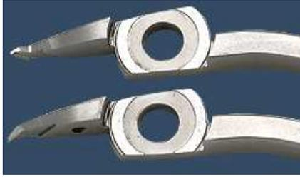
**Hardened nut of alloy steel & extended cross-sectional area** anchors the joint against movement under the cutting load. Precision machining of the nut insures perfect alignment of the two cutting edges.
