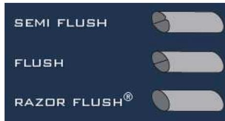
What is Razor Flush®? This is the name Tronex uses for the edge finish and anti-dulling protection on cutter models that cut exceptionally flush.
