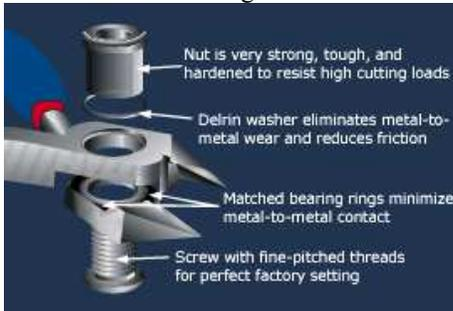
**Bearing rings** are machined into the bearing surface of each cutter body. The rings face each other as the two halves are brought together. In cutter operation, over perhaps hundreds of thousands of cycles, the two halves only bear and move against each other over the very limited area of the
