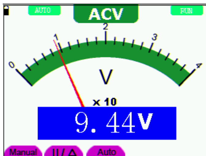
figure 26: AC Voltage Measurement
