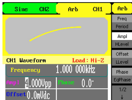
Figure 1-12 Arbitrary waveform Signal Display Interface As shown in Figure 1-12, the default sine signal parameters are: 1kHz frequency, 4.0 Vpp amplitude and 0mVdc offset.
