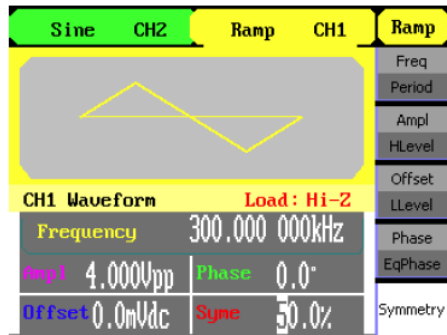
Figure 2-9 Ramp Parameter Display Interface
