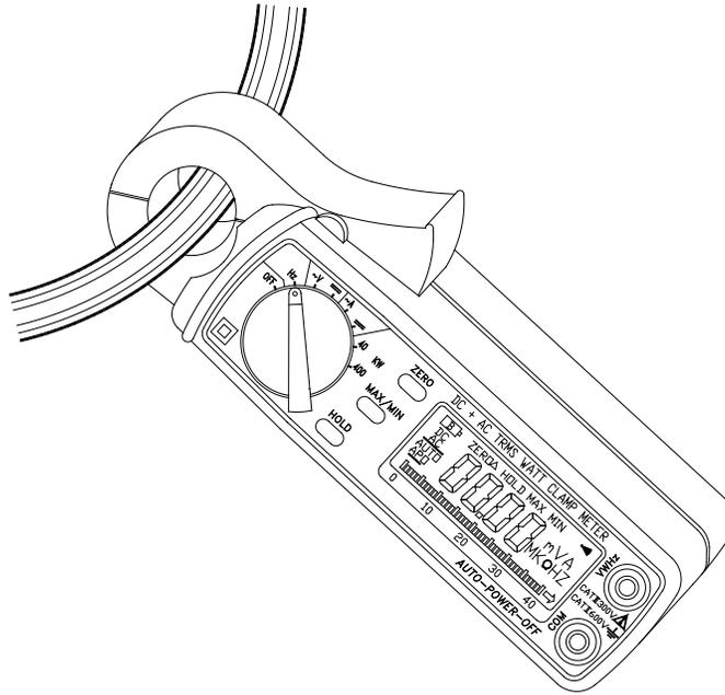
**WARNING:** Make sure that all the test leads are disconnected from the meter's terminals for current measurement.
