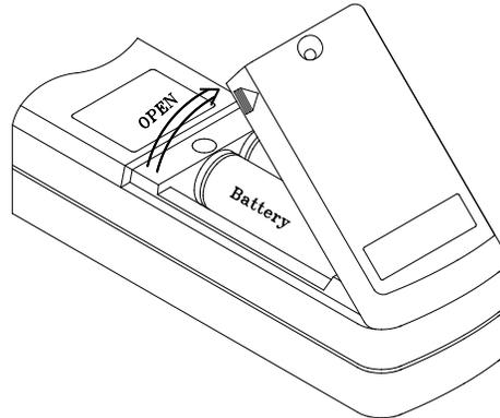
When the low battery symbol is displayed on the LCD, replace the old batteries with two new batteries.
