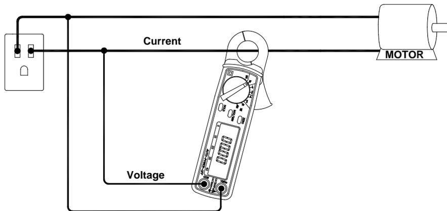
1. Connect the test leads to the voltage source in parallel with the load.
