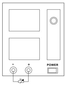
Load is connected as shown above. After the unit is switched on, output current will be indicated by LED, LCD or analog meter (2), and output voltage indicated by LED, LCD or analog meter (1). The unit may be overload or short-circuit. You should adjust the load to have the unit working properly.
