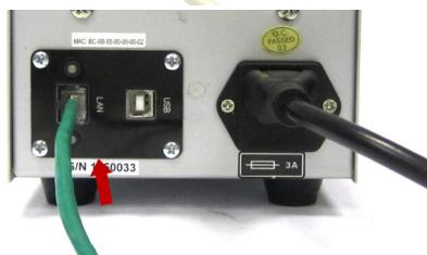
Connect the device **LAN** port with the local network using Ethernet cable.
