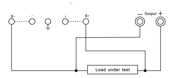
Attention: Disconnect the installed S- and S+ shorting wires when using the sampling connections.
