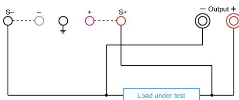
Attention: Disconnect the installed S- and S+ shorting wires when using the sampling connections.
