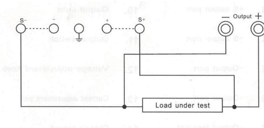
**Attention:** Disconnect the installed S- and S+ shorting wires when using the sampling connections.
