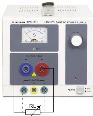
Load is connected as shown above. After the unit is switched on, output voltage indicated by Analogue meter (1). The instrument can supply Max. 10000VDC when connect the load in terminal(2) and (4), but in some situation that safety is all-important, connect the load in terminal(2) and (3) is proper.
