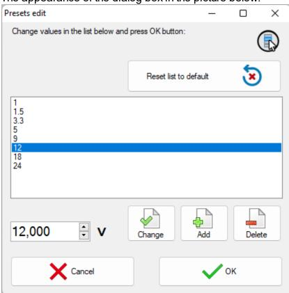
The list of presets (shortcut buttons) is a list of Voltage or Current values, which can be set on the device "with one touch". In dialogue editing presets in addition to the list itself, the program displays the following buttons:
