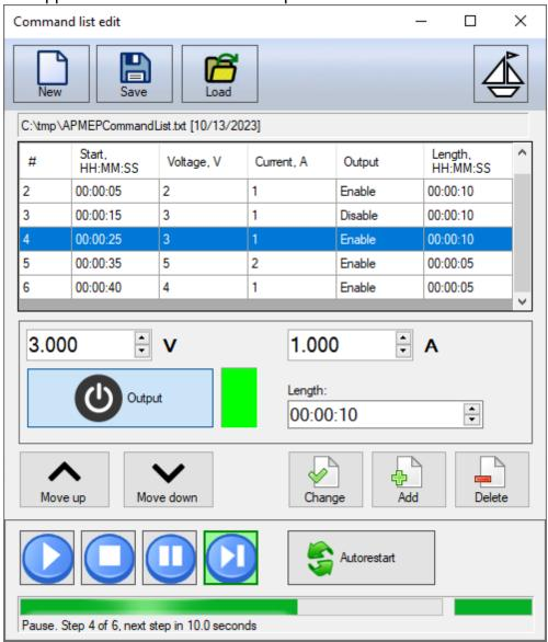
The panel makes allows the user to specify a list of commands that will be automatically sent to the device sequentially.
