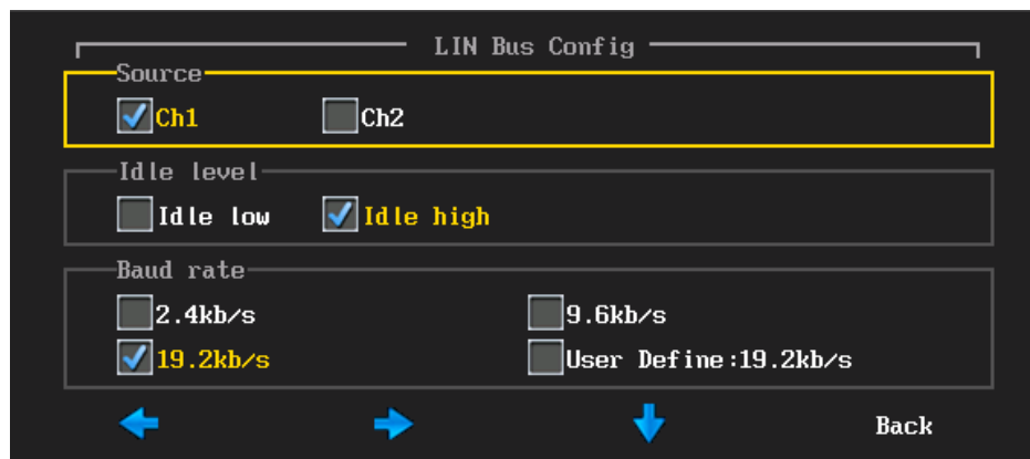
Picture 4-7 LIN bus configuration menu
