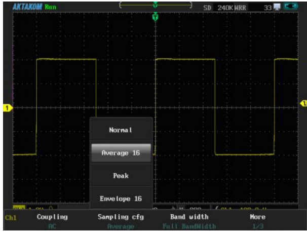
Picture3-6 average 16 sampling config
