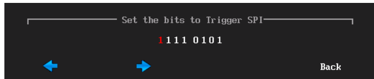
Picture 4-17 SPI matching bit settings menu
