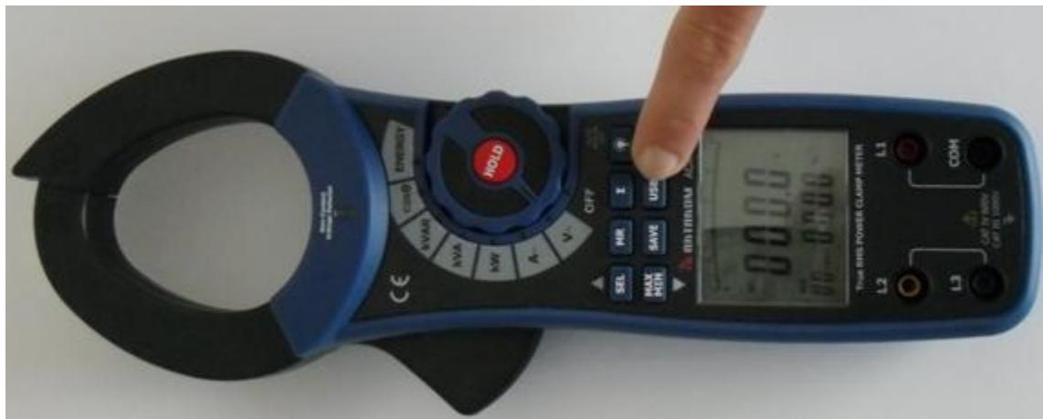
Please press USB button to turn on the USB function, the icon appears on the LCD. When you have finish press the button again to return to normal operation.
