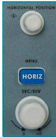
Fig. 4-12 Horizontal Control Zone
