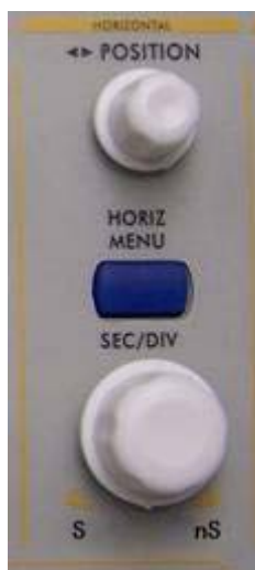
Fig. 4-10 Horizontal Control Zone
