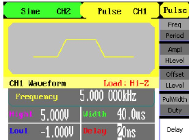
Figure 3-4 Pulse Waveform
