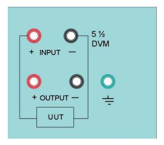
Diagram 4.6 Measuring the Voltage of the Instrument under Test
