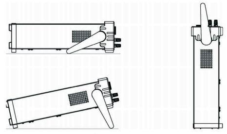
Diagram 3.3 Power Supply Viewing Positions
