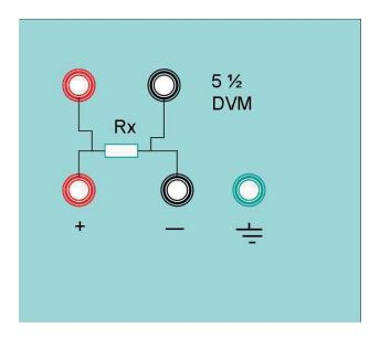
Diagram 4.5 Milliohmmeter Measuring Resistance
