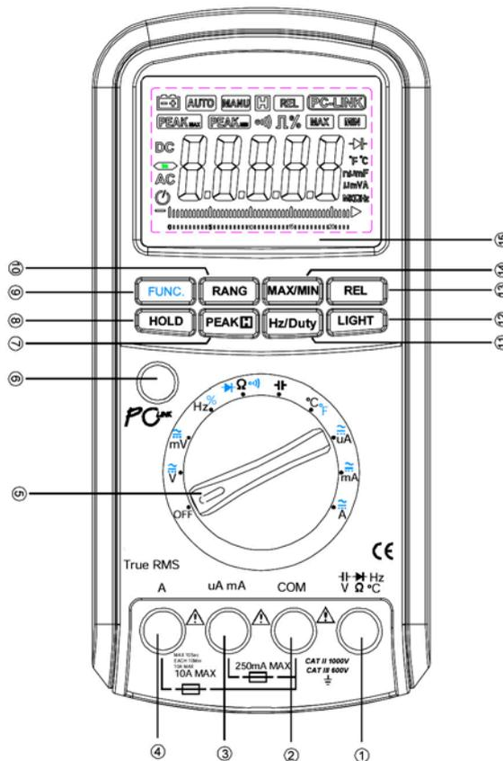
**(1) V/ $\Omega$ / $^{\circ}$ C/CAP/DIODE/Hz end**
