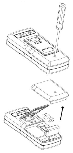
Remove any test leads before removing the battery cover. Users will see the battery and fuses. Replace the old ones with new battery or fuses. Replace the battery cover.
