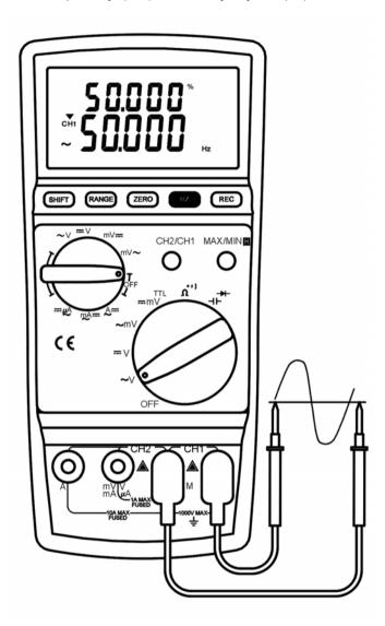
If the rotary switch is set at either position of V, mV, A, mA, or  $\mu$ A, the measurement of frequency and duty cycle can be selected by pressing the SHIFT button.
