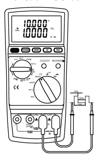
Users set the rotary switch at DC mV of channel 1. If the SHIFT button is pressed, the DMM will perform measurement of frequency and duty cycle of a TTL signal
