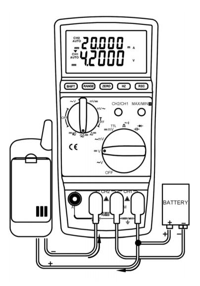
This unit can perform dual channels measurement of voltage and current at the same time. The internal circuit will multiplex between two channels. It is very useful when users need to observe the relationship between voltage and current in a circuitry.
