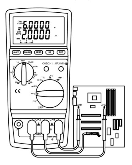
This unit can perform dual channels measurement of voltages at the same time. The internal circuit will multiplex between two channels. It is very useful when users need to observe the relationship between two signals in a circuitry similar to dual channels DSO.
