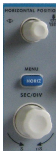
Fig. 4-13 Horizontal Control Zone
