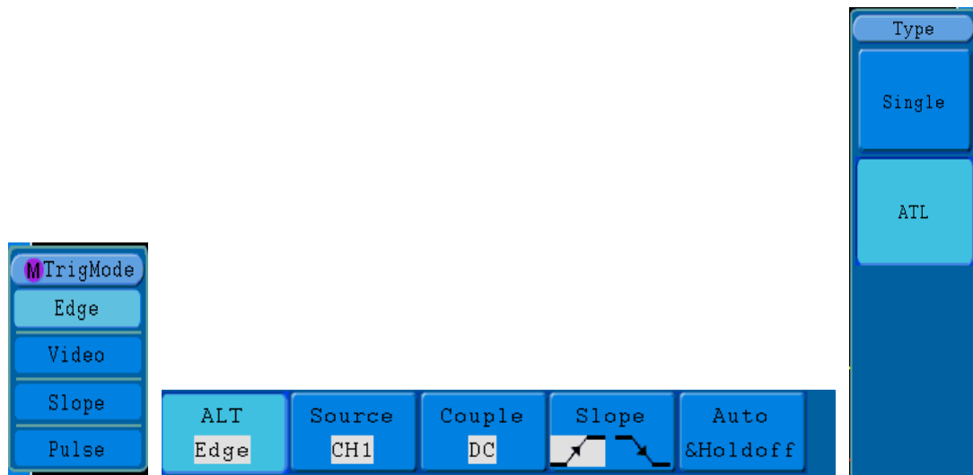
Fig.5-21 Alternate trigger (Trigger Type: Edge) Menu
