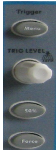
Fig.4-14 Trigger Control Zone
