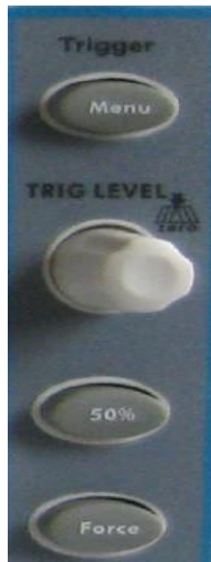
Fig.4-14 Trigger Control Zone
