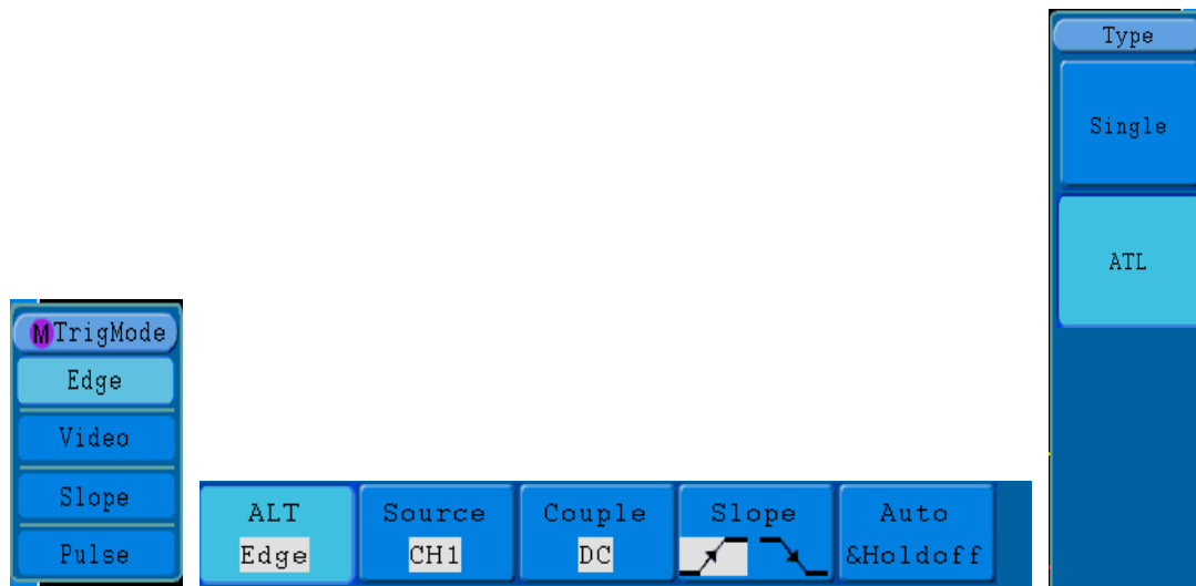
Fig.5-21 Alternate trigger (Trigger Type: Edge) Menu
