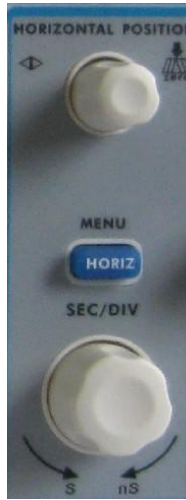
Fig. 4-13 Horizontal Control Zone
