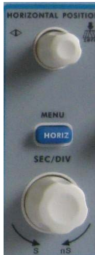
Fig. 4-13 Horizontal Control Zone
