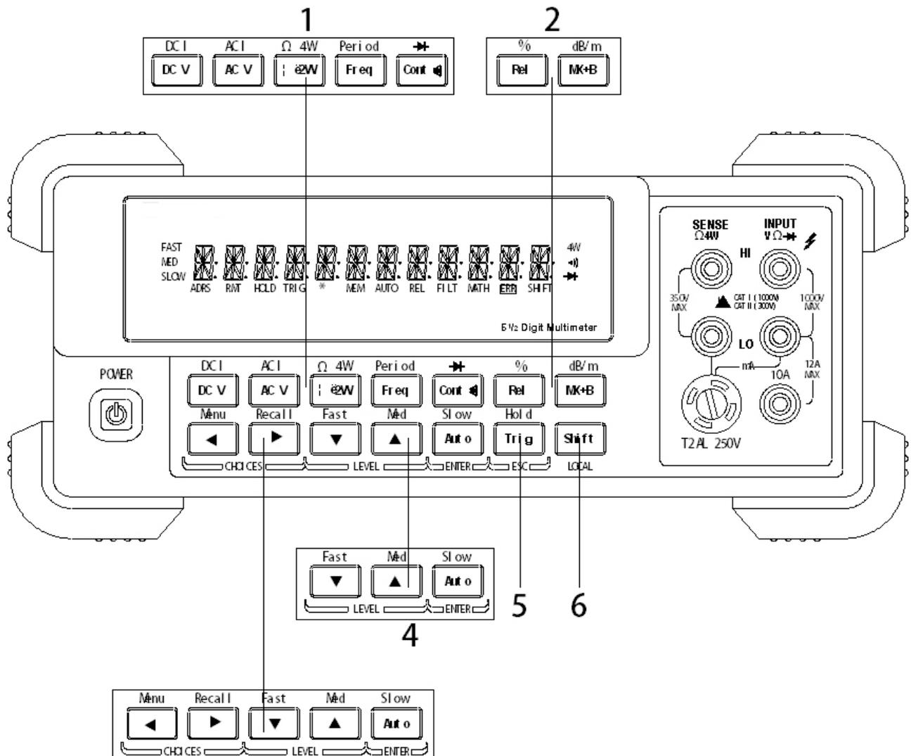
Figure 2-1 DMM Front Panel
