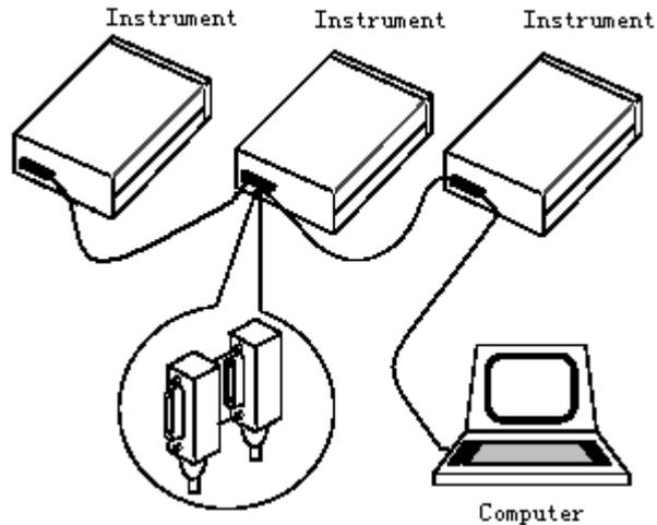
Figure 5-4 Typical GPIB System Interconnection
