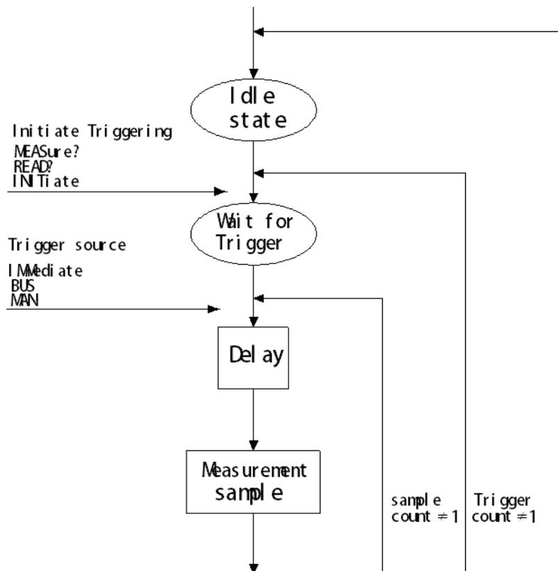
**Figure 4-2 Trigger model**
