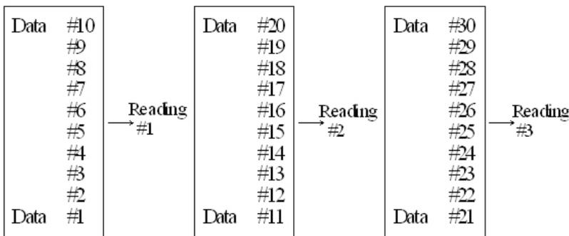
**Figure 4-1 Moving average and repeating average filters**
