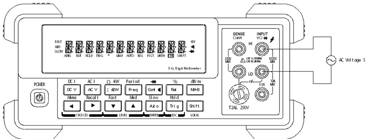
Input Impedance = 1MΩ in parallel with <100pF
