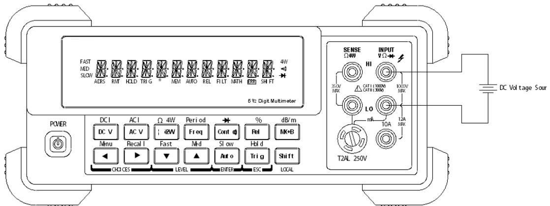
Input Resistance = 10MΩ on 1000V and 100V ranges;
