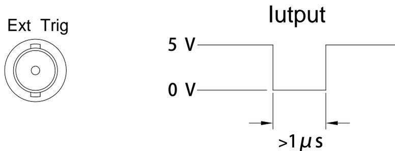
Figure 4-3 Trigger model
