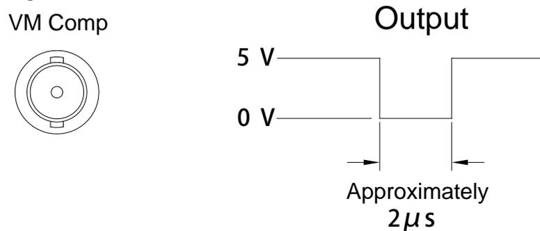
Figure 4-4 Trigger model
